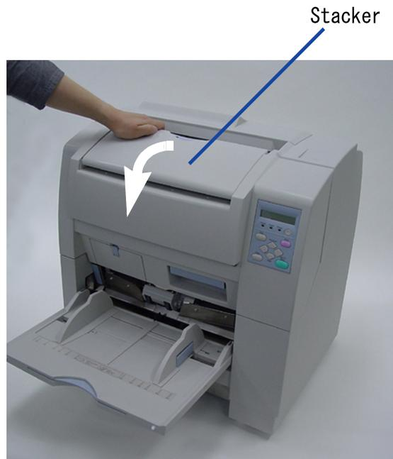
4) Wipe the following parts using a cloth moistened with Cleaner F1 or isopropyl alcohol.
