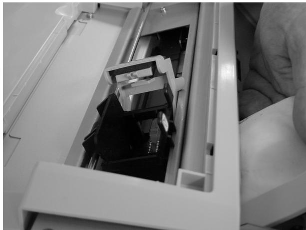
5) Lift the Upper transport unit slightly to release the safety lock and then lower and close the transport unit slowly.
