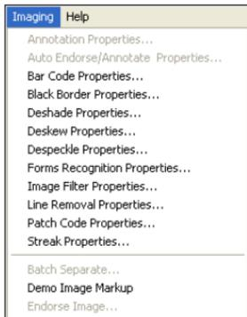
Each of these options displays a setup dialog box for image processing and cleanup features. You can use these dialog boxes to enable one or more of the features and select the desired settings. Units for some of the measurements that you can select are controlled by the preferences set with the Units option on the File menu.
