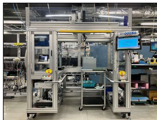
Appearance of the Developed Shipping Inspection System
